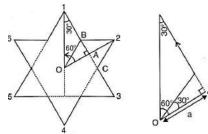
Direction of magnetic field at O due to each segment is same.
